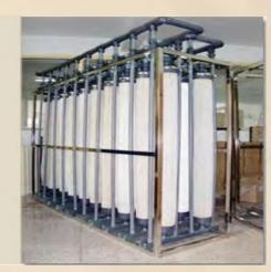
The Membrane Bio Reactor (MBR) is the technology of membrane separation combining with traditional sewage biology treatment Ιt reinforces tech. the biological treatment on sewage treatment and recycling technology, it is also called membrane separation activated sludge treatment. MBR holds the activated sludge and big molecule
